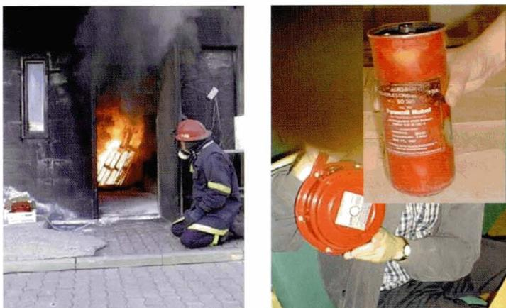
Figure 3: Pyrotechnical extinguishing grenades at a demonstration
