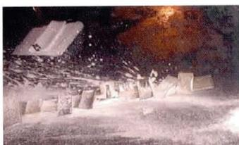
Figure 7: Test set with 13 different museum objects is sprayed with aqueous film forming foam following exposure to smoke from a Class A fire at about 200 °C
