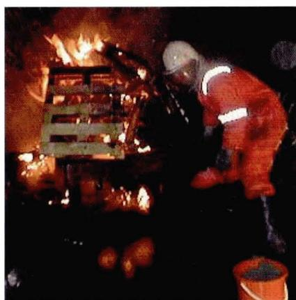
*Figure 11: Sand applied in extinguishing performance test. The sand used was too wet for successful application.*
