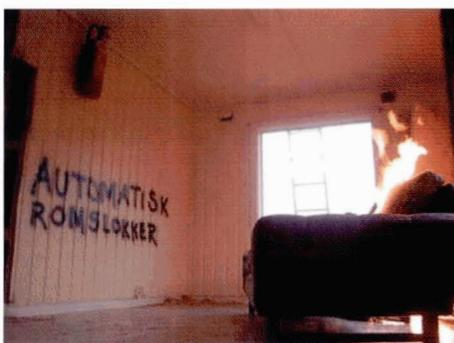
Figure 12: Realistic performance test of ceiling category automatic extinguisher (COWI AS)
