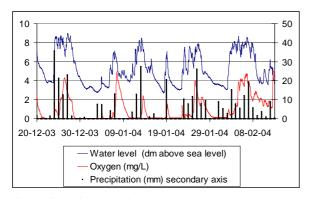
Example of results from dipwell MB4, where porous deposits give instant responses after rainfall, resulting in increased water-level and oxygen content. The logger is situated at -1.3 m asl, or 2 m below the average groundwater level.
