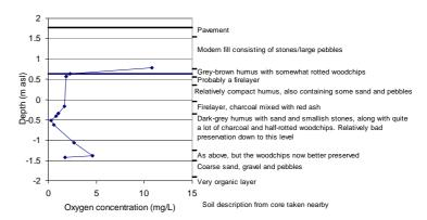
Oxygen profile measured directly in undisturbed soil by Ev Kretschmar, University of Göttingen. Soil surface is at 1.77 m above sea-level (asl) and blue line indicates the groundwater level at time of recording.
