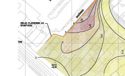
Map of Bryggen showing measured settling rates for the buildings and ground surface in mm/year. Orange line indicates sheet piling between the old wooden buildings and the excavated area (now occupied by new buildings).
