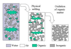
Drainage may lead to settling through a physical process as well as by the decomposition of organic matter.
