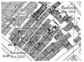
Map of Bryggen showing position of dipwells (MB1-8) and test excavations. The hotel was built in 1980 on the site excavated during the 1950s and -60s.
