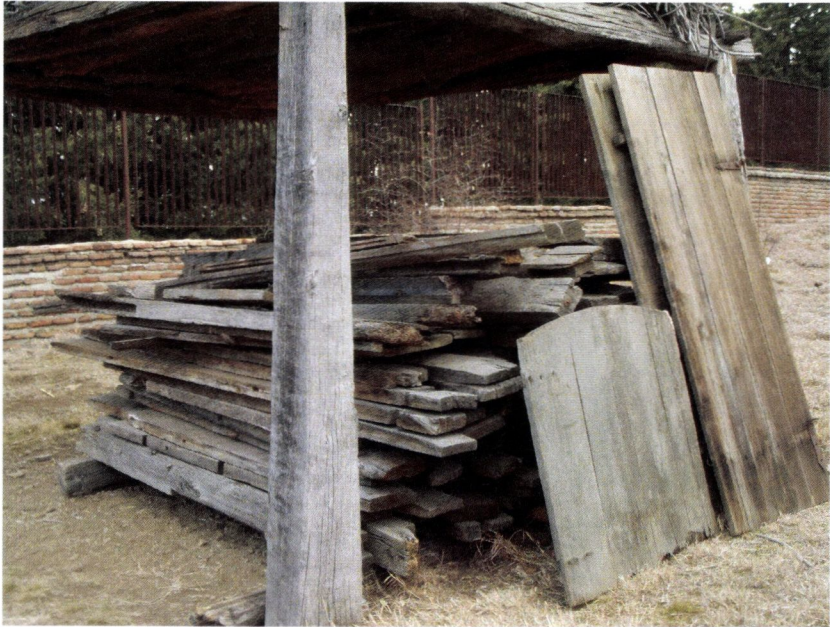
Applicable and restorable timber of the Goraberejouli house
