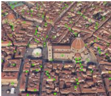
Monitoring of the Florence city center by means of radar satellite interferometric techniques exploiting Copernicus Sentinel-1 constellation.
