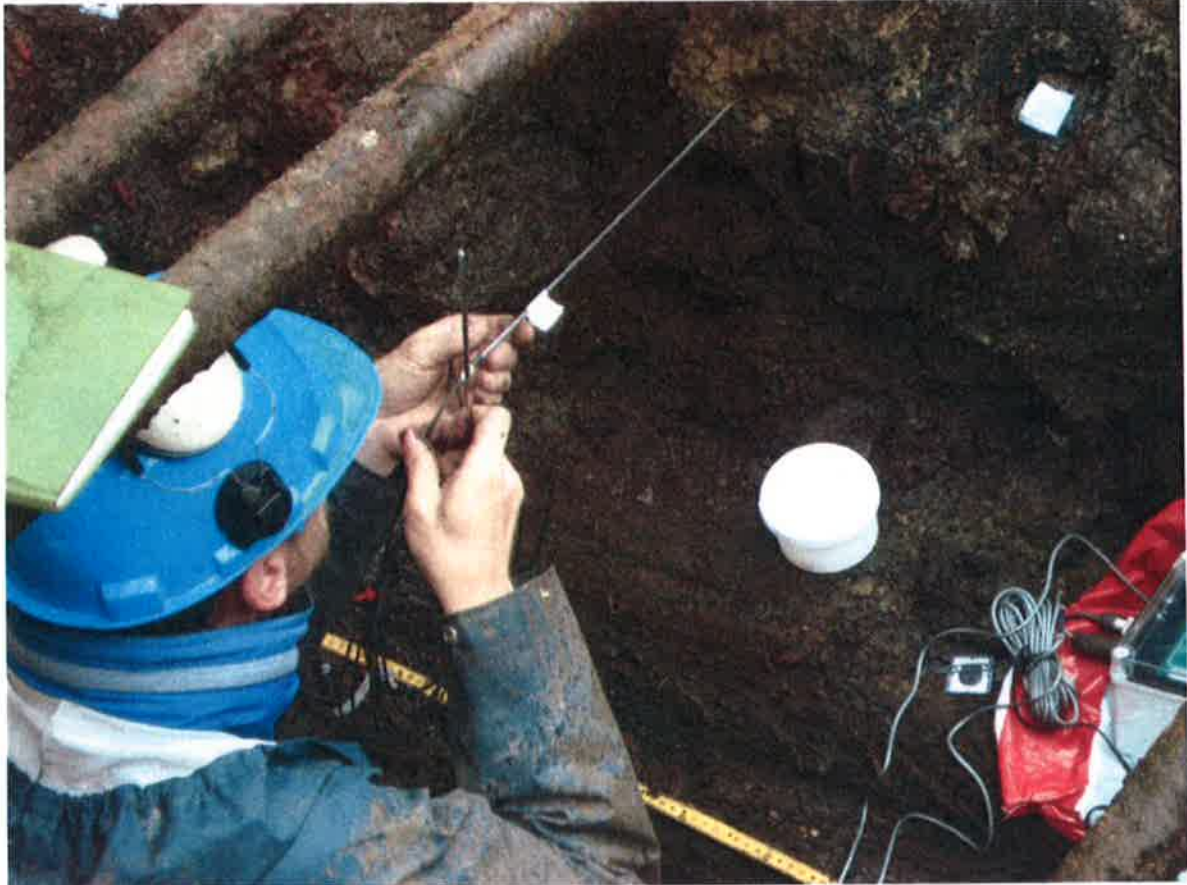
Figure 4: Installation of the oxygen sensor in the profile.
