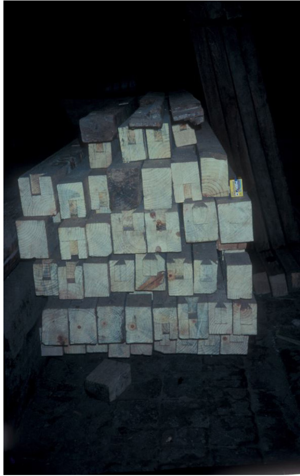
Figure 6.2 Softwood used in Nepalese preservation work. The width of the annual rings is approximately one centimetre. The amount of heartwood was almost negligible.
