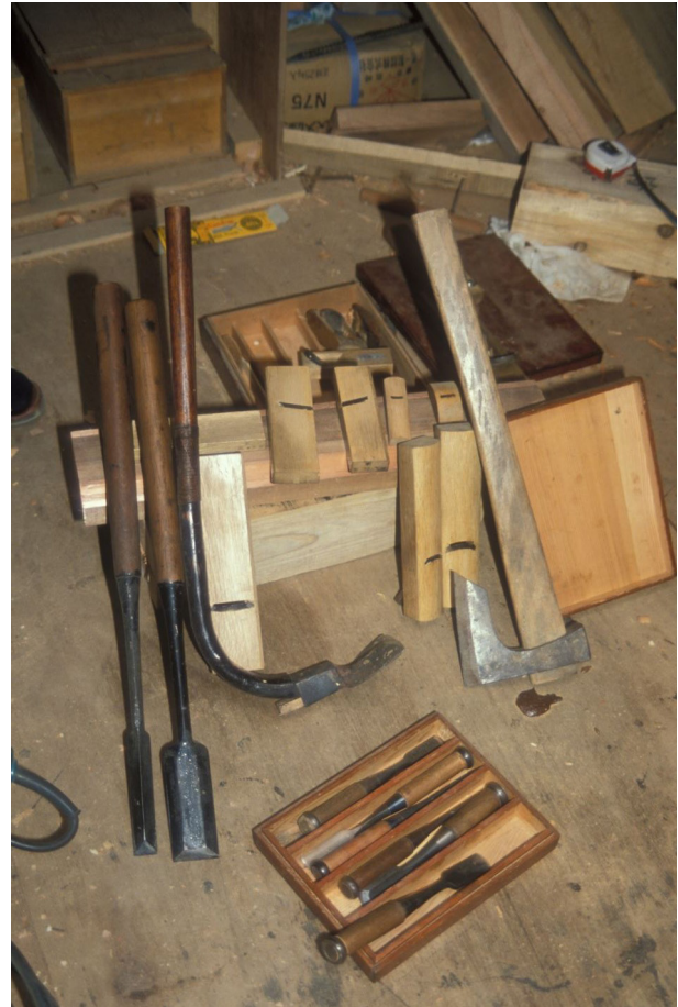
Figure 5.1 Tools used by carpenters in the repair of the three-storied Oyama-dera pagoda, Japan in 1989: adze and axe; two kinds of chisels - used by pushing ( left ), or by striking ( tool box in centre ); planes - left , a common plane; centre , rebate planes; right , molding planes.
