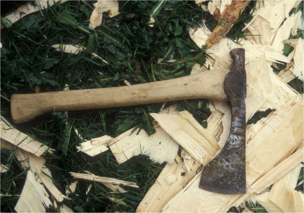
Figure 1.2 A carpenter's axe used for "sprett-telgjing".
