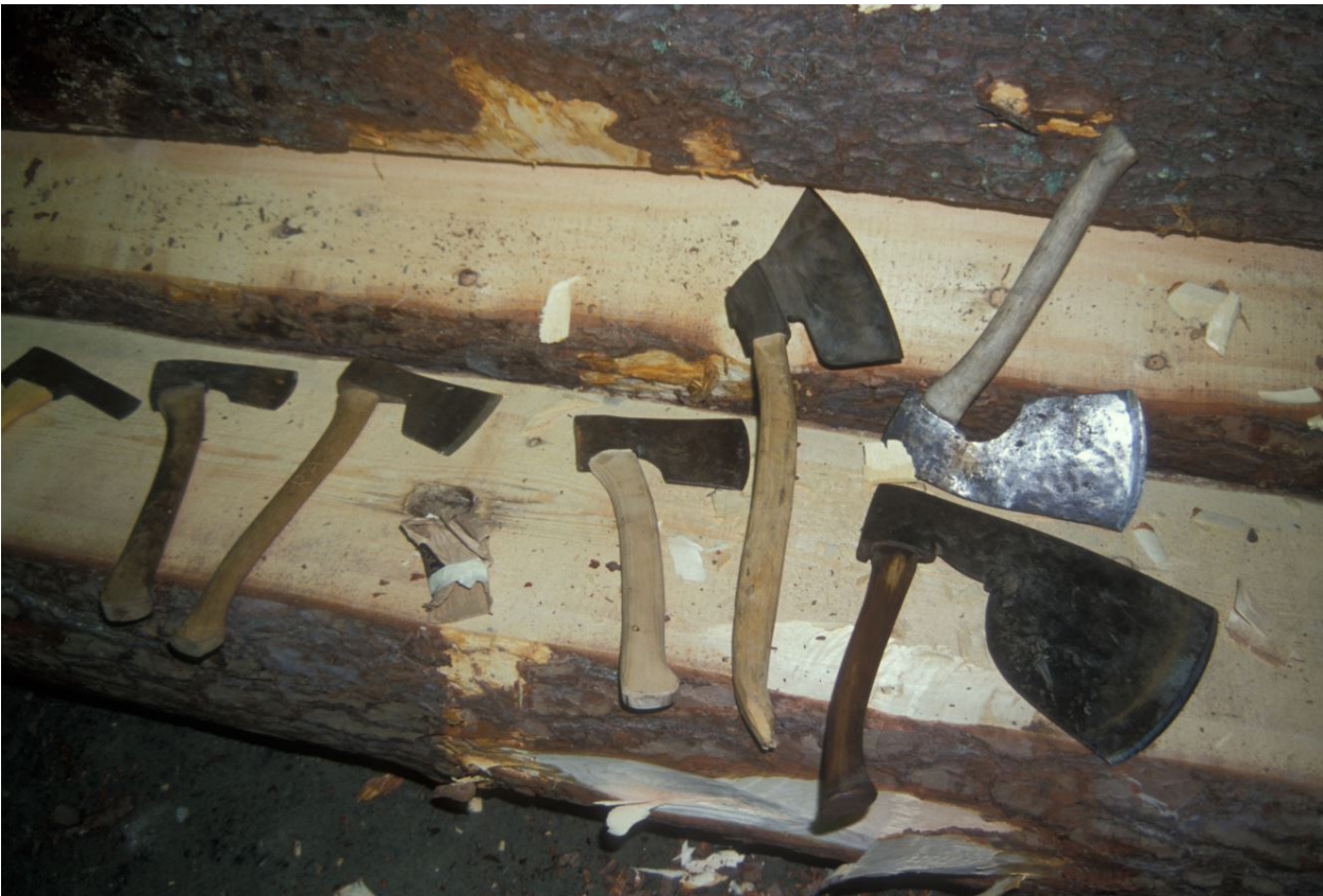
Figure 5.2 Axes used by Norwegian carpenters in the repair programme for medieval timber structures 1991-1996.
