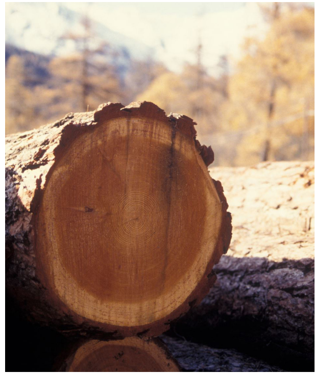
Figure 8.2 The end section of a larch log ( Larix decidua ). The heartwood covers almost the whole cross-section; there is only a narrow outer ring of sapwood.
