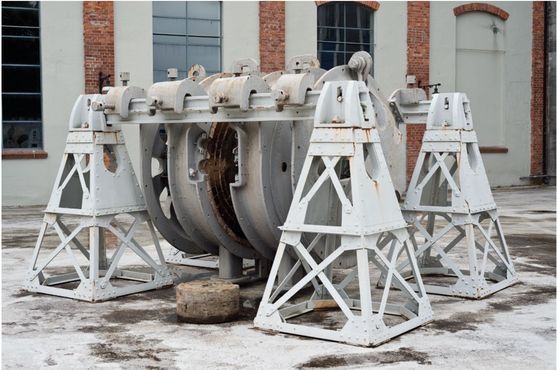
Fig. 51 Electric Arc Furnace, Notodden. Photo: Per Berntsen
