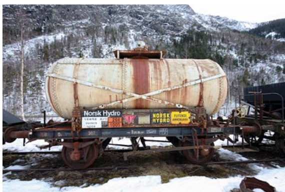
Tank wagon for ammonia. Photo: Eystein M. Andersen
