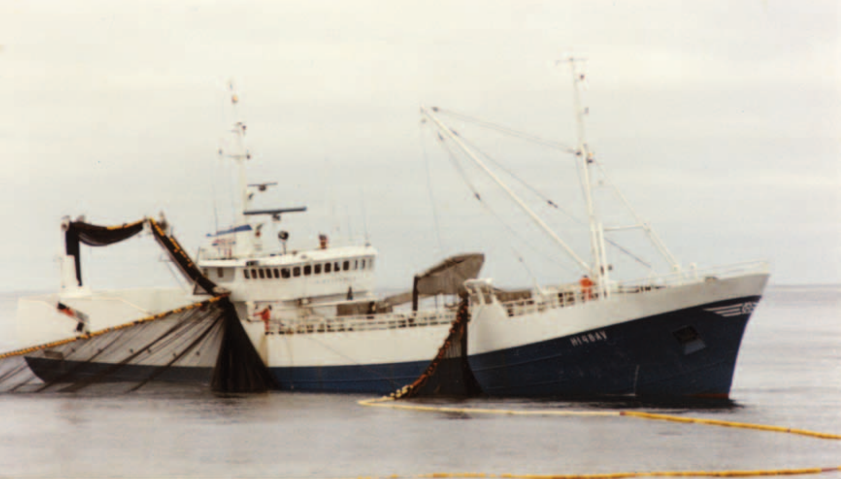
The ring net boat hauls in an enormous ring net using a power winch. From the 1960s most catches of herring, mackerel, capelin, and blue whiting were taken with such highly efficient fishing boats. Photo: Norwegian Fisheries Museum
