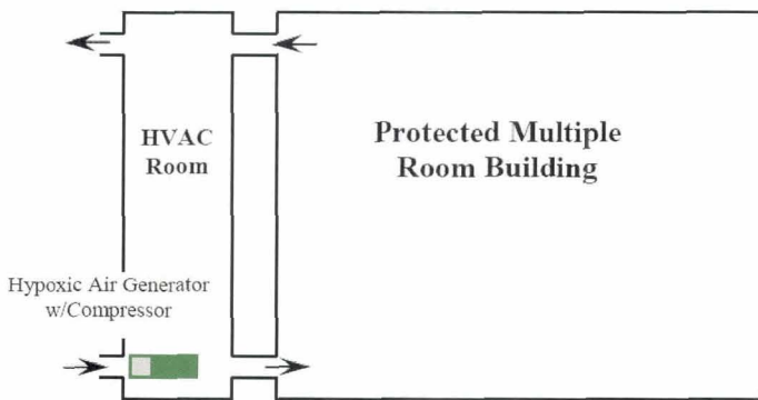
FIRE PREVENTION AND EXTINGUISHING Hypoxic Air Venting
