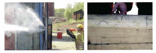
*Figure 13: Piercing high pressure water mist nozzle during performance demonstration. Log wall is penetrated. Note 2 mm diameter tracks by penetrations at joints.*
