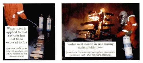
*Figure 5: Water mist extinguishers applied to material samples not exposed to fire, and in extingusihning test.*
