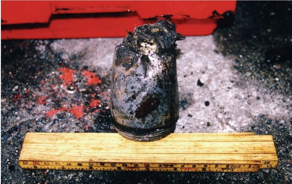
Lower end of 54 mm core sampler damaged on encounter with well-preserved timbers in archaeological deposits (photo: Dunlop, NIKU).
