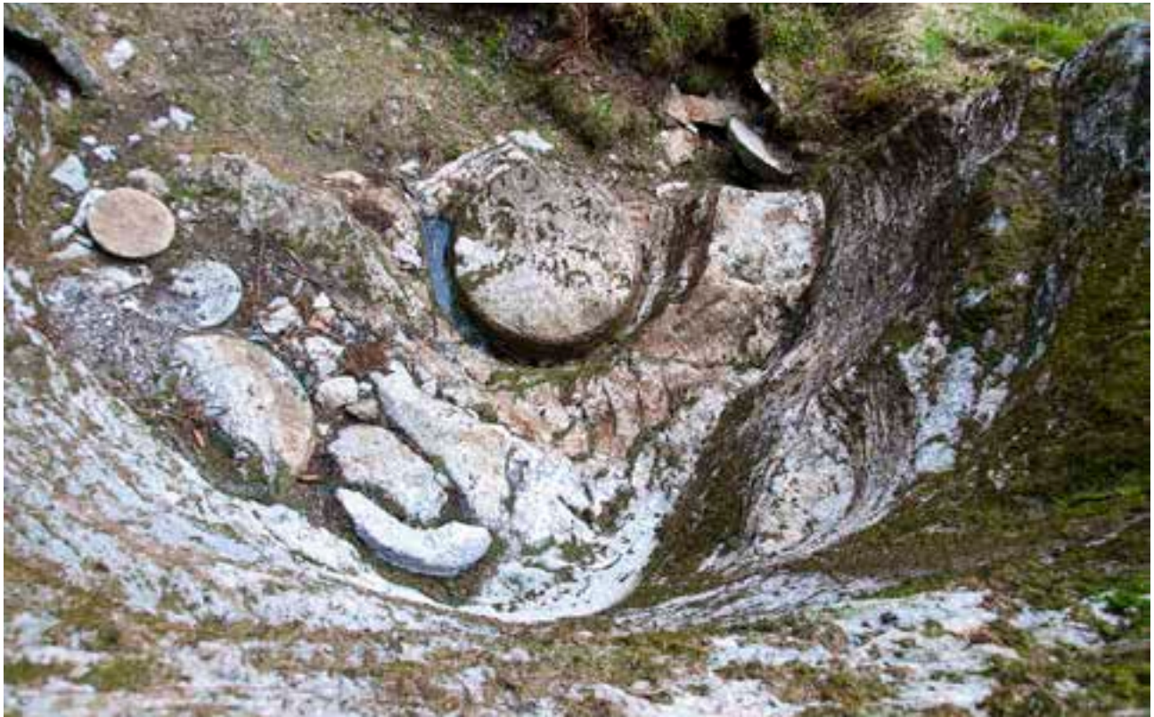
FIGURE 2.54 Unfinished millstone still attached to the rock ©Kim Soderstrom/Jorgen Magnus, Directorate for Cultural Heritage.
