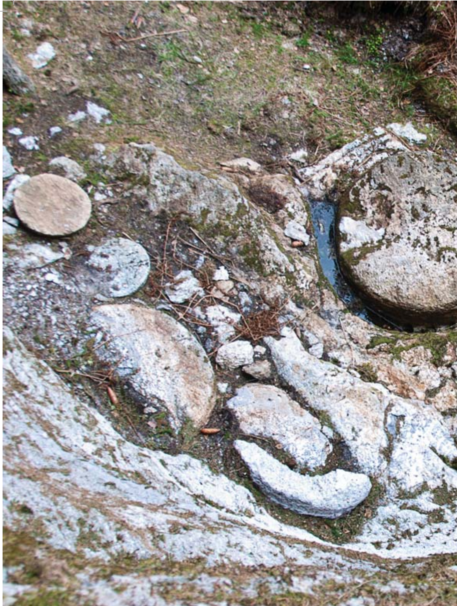
Figure1: Deep quarry with production of quernstones and millstones located in Millstone Park, Myklebust . Photo: Kim Söderström and Jørgen Magnus, Directorate of Cultural Heritage
