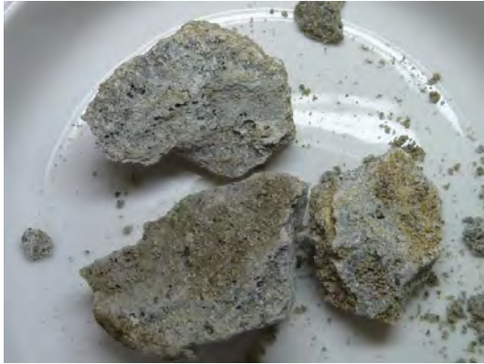
Plate No. 1: View of the mortar sample as received, placed in an evaporation dish and weighed in preparation for moisture content determination.
