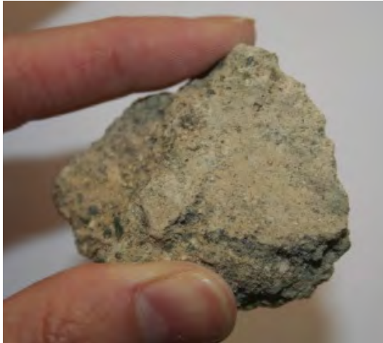
Plate 3. The flat, litaunce-rich surface of one piece of the mortar sample.
