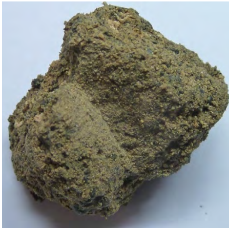
Plate 3. Piece of mortar, in the as received (saturated) condition, submitted for XRD analysis.
