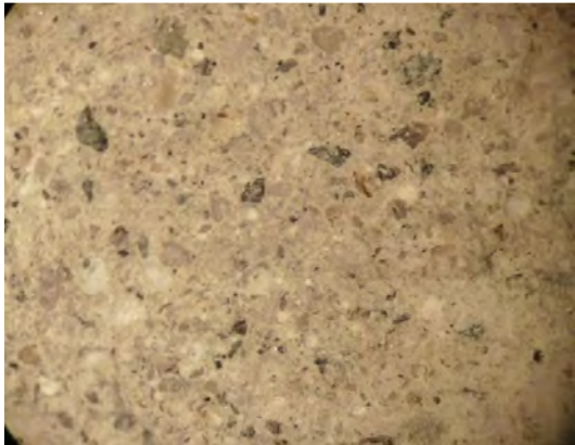
Plate No. 3: View through the microscope showing the dense fabric, with angular aggregate particles. Small round entrained air bubbles can be seen, which are infilled with Portlandite crystals.
