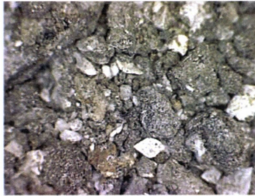
Plate 4. Close up of some of the mortar fines received (c. x30 magnification).
