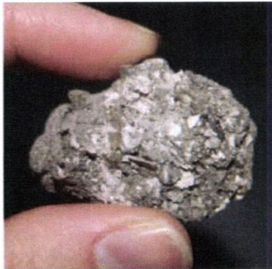
Plate 3. A face of the sample rich in lime inclusions at a higher magnification.
