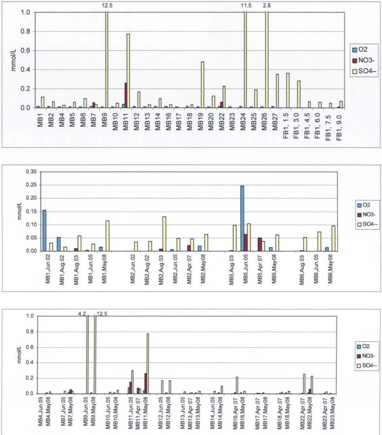
Figure 5: Concentrations of different oxidants in the dipwells in May 2008 (upper diagram) and as time series (lower 2 diagrams). Oxygen wasn't analysed in May '07, and in May '08 there is a systematic pollution or bias of approximately 0.02 mmol/L. For results in mg/L the numbers in mmol/L must be multiplied by 32.00 for oxygen, 14.01 for nitrate (to give mg N/L), and by 96.06 for sulphate (to give mg SO 4 2- /L)
