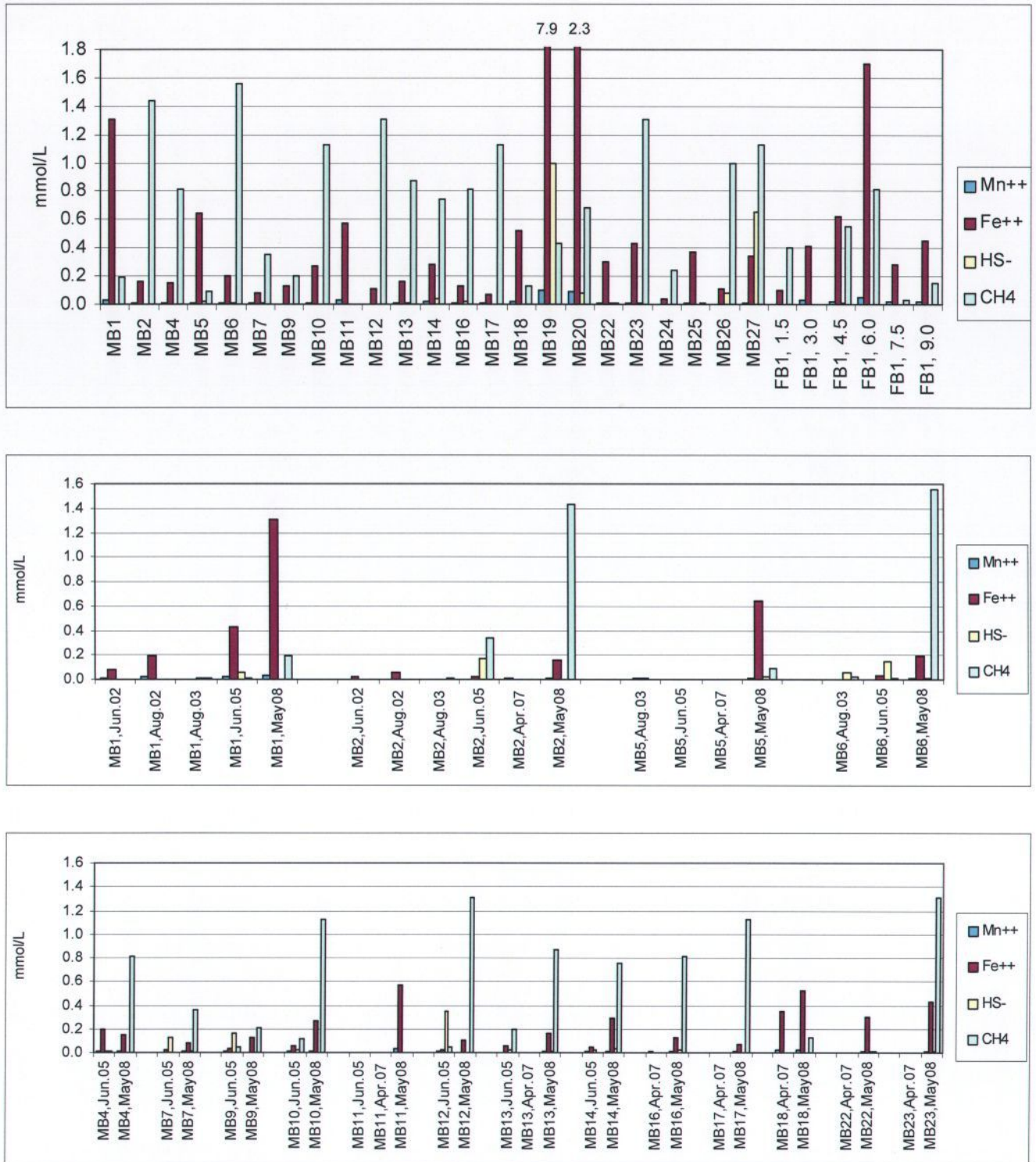
Figure 6: Concentrations of different reduced species in the dipwells in May 2008 (upper diagram) and as time series (lower 2 diagrams) – NH 4 + is shown in Figure 4. For results in mg/L the numbers in mmol/L must be multiplied by 54.94 for manganese, 55.85 for iron, 32.06 for sulphide (to give mg S/L), and by 16.04 for methane (to give mg CH 4 /L). Sulphide wasn't analysed in Apr. '07, and in May '08 the results for MB2, MB9, MB12 and MB24 were reported as "too high" for the analytical method applied. Methane was only measured in August '03, June '05 and (with a dedicated sampling technique to avoid loss) in May '08. No sample was taken for methane or sulphide from FB1 (3.0 m) in May '08.
