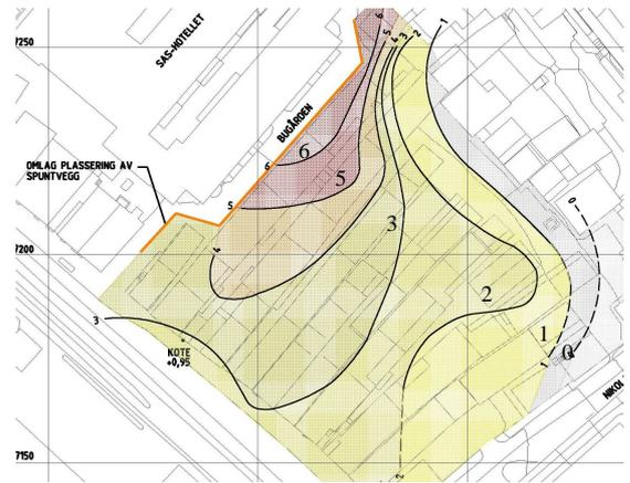
Map of Bryggen showing measured settling rates for the buildings and ground surface in mm/year. Orange line indicates sheet piling between the old wooden buildings and the excavated area (now occupied by new buildings).
